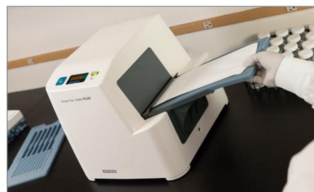
5. Immediately seal the tray using the Quanti-Tray\* Sealer PLUS.
