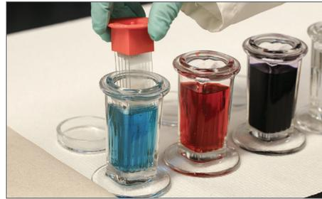
2. Dip the slide holder 3 times in fixative to coat the slides. Then immerse the slide holder in fixative for 30 seconds. Tap the slide holder gently on absorbent material to absorb any extra fixative.
