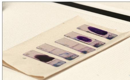
6. Remove slides from the slide holder and allow to air-dry or use a fan.
