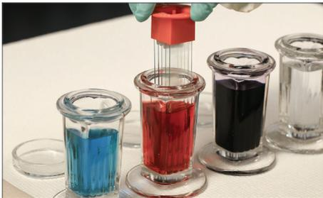
3. Dip the slide holder in red stain 3 times to coat the slides. Then immerse the slide holder in red stain for 5 seconds. Tap the slide holder gently on absorbent material to absorb any extra red stain.
