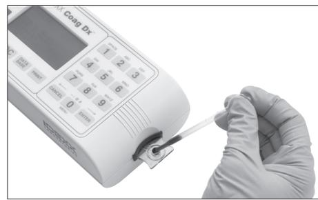
**Figure 4-10:** Add sample to center of well
