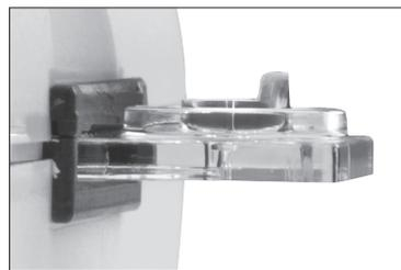
**Figure 4-12:** Insufficient sample
