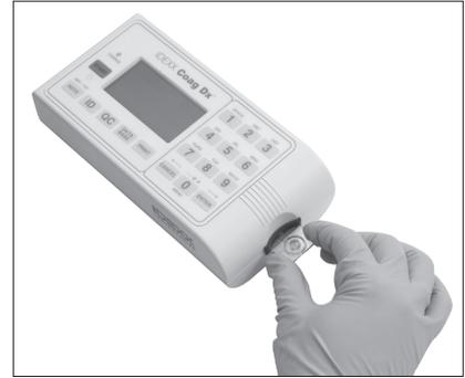
**Figure 4-1:** Insert Coag Dx PT or aPTT cartridge
