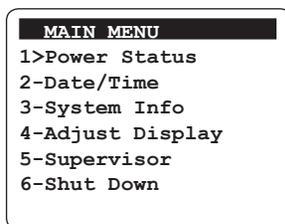
To execute a command on any menu, press the applicable number key for that command. For example, on the Main menu, press **6** to shut down the system or press **3** to display system information.
