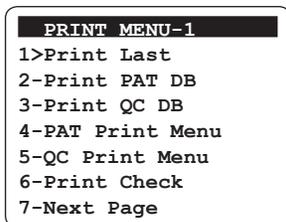
3. Press **6** to print an ASCII character set to the attached printer to verify that the printer port functions properly.
