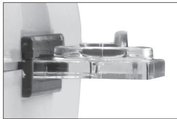
**Figure 4-4:** Insufficient sample
