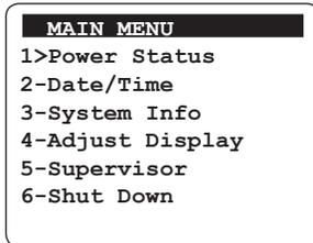
2. Press **6**. The analyzer shuts down.
