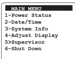
2. Press **5** to display the Supervisor menu and enter the personal identification number (PIN) to access this menu. If a PIN has not yet been assigned, **press and hold the Enter** key to access the menu.
