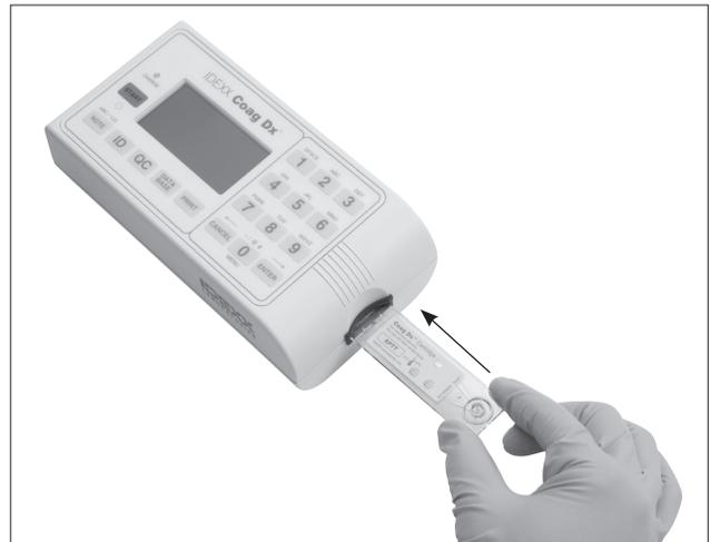
**Figure 3-1:** Insert cartridge, label facing up
