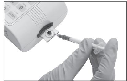
**Figure 4-2:** Add sample to center of well
