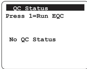
3. Press **1** to initiate the EQC process. The test chamber warms to 37°C ±1.0°C (98°F ±1.0°F) and the EQC test begins. The results are displayed while the test is progressing.
